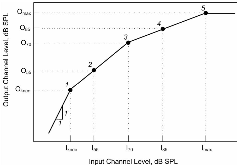
**Figure 8.** Example I/O characteristic for one channel of a compression hearing aid.
