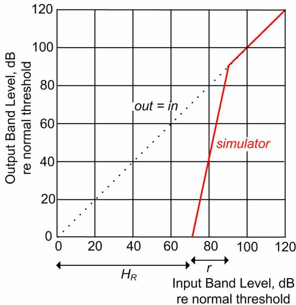
**Figure 3.** An example I/O plot for one simulator band showing a recruiting hearing loss  $H_R = 70$  dB with a recruitment range  $r = 20$  dB.
