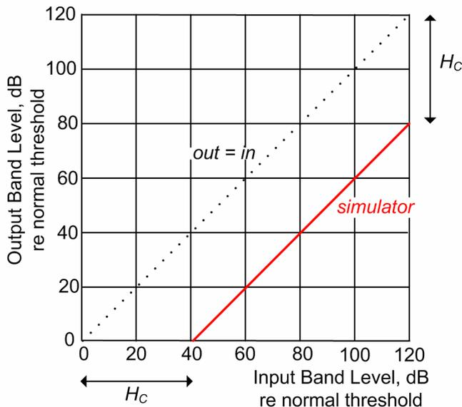
**Figure 2.** An example I/O plot for one simulator band showing a conductive hearing loss of  $H_C = 40$  dB.
