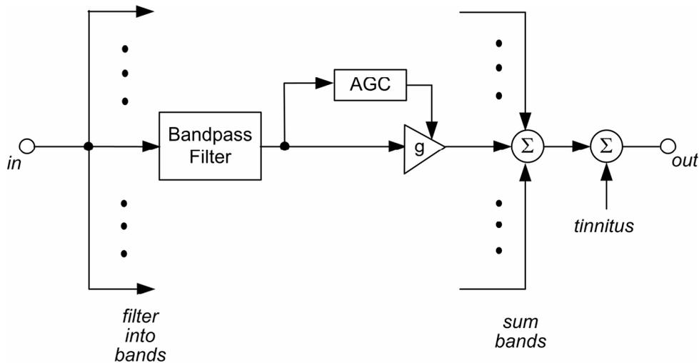
**Figure 5.** Block diagram showing the signal processing in one band of the hearing loss simulation.
