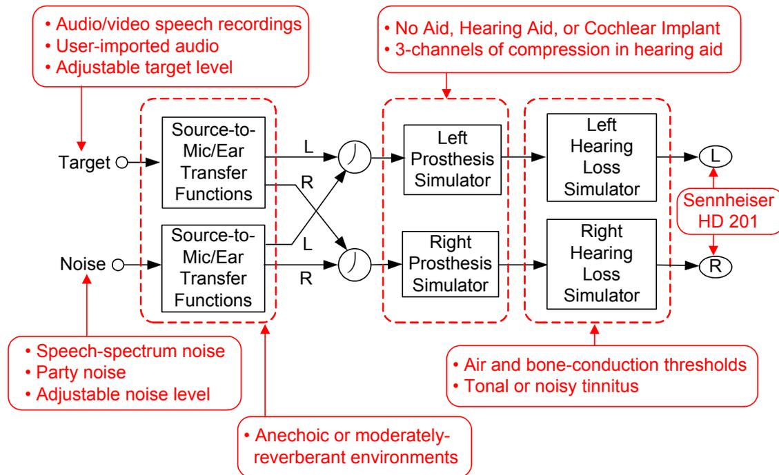
**Figure 1.** Block diagram showing the main signal and signal-processing components of the HeLPS simulation.
