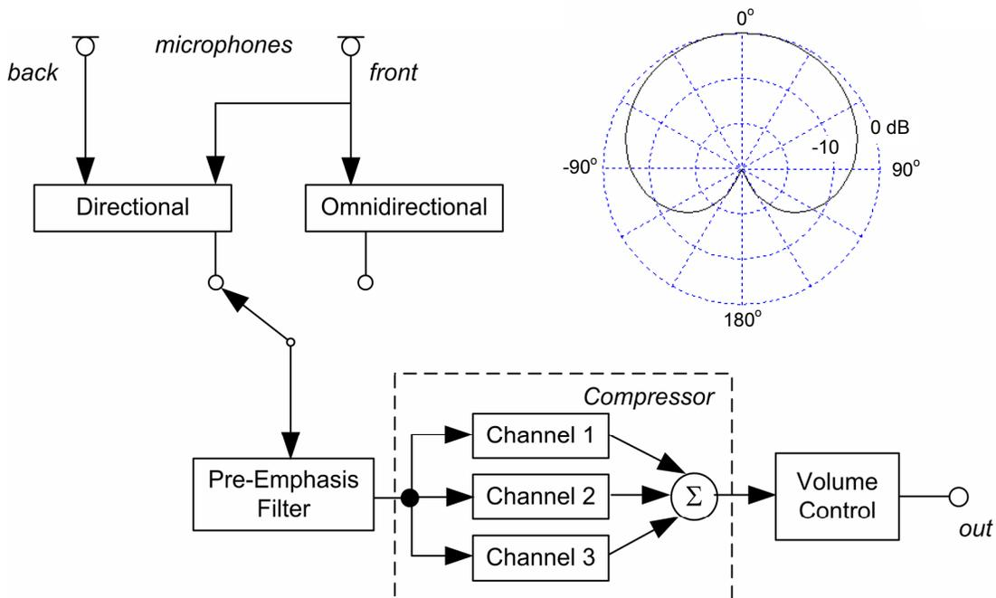
**Figure 6.** Block diagram of the prototype hearing aid implemented by HeLPS.
