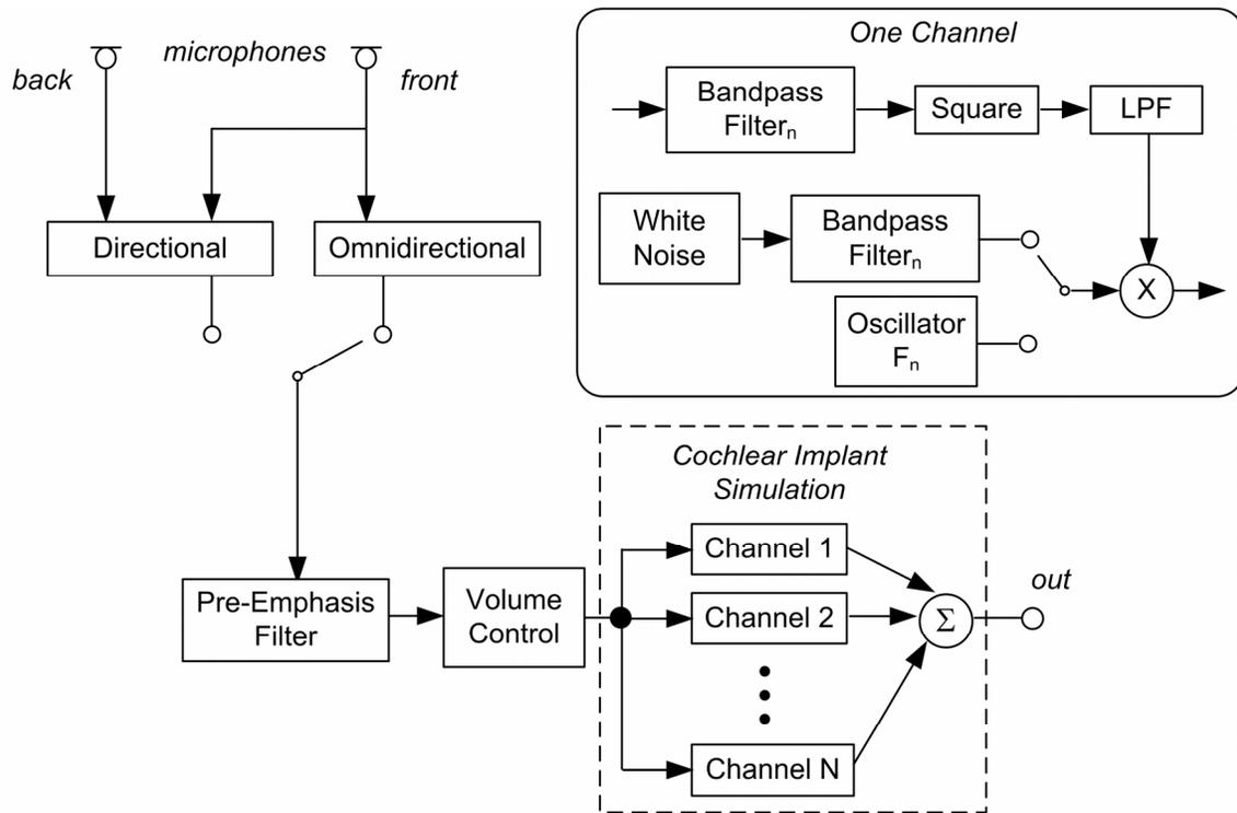
**Figure 7.** Block diagram of the prototype cochlear implant simulation. The processing performed within any one channel of the implant simulation is shown in the inset.
