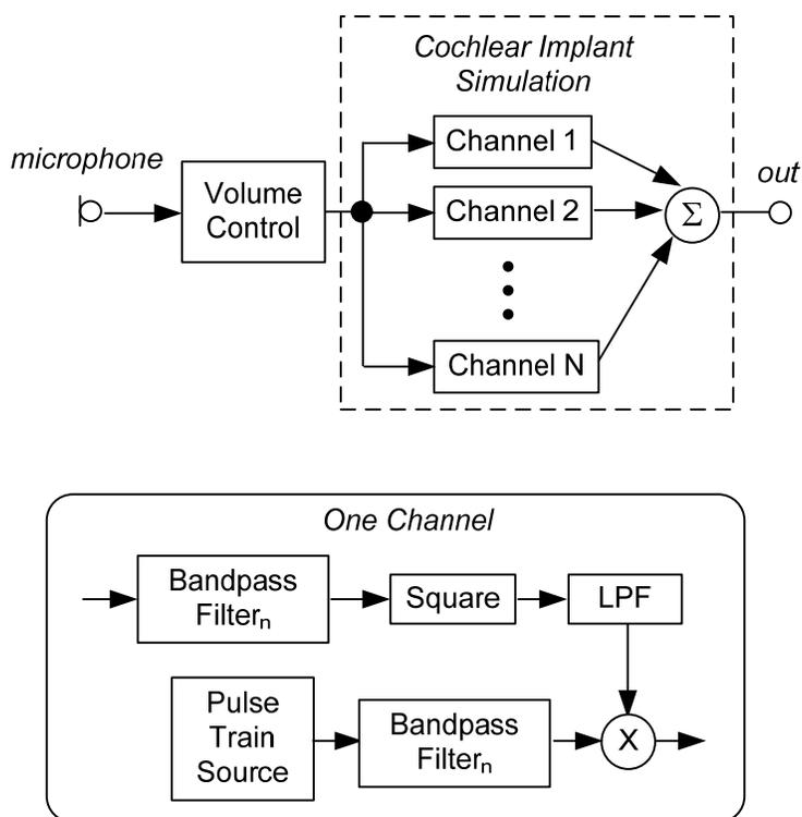
Figure 8. (Upper) Block diagram of the prototype cochlear implant simulation. (Lower) The processing performed within one channel of the simulation.
