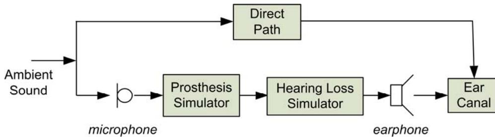
Figure 2. Diagram showing one channel of an immersive simulator (lower branch) along with the direct acoustic path (upper branch).
