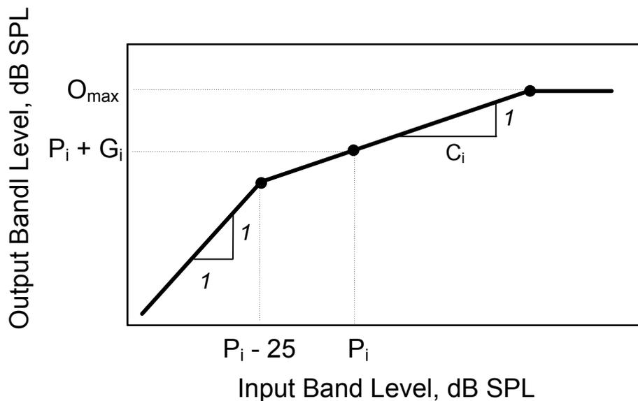
Figure 7. Example I/O characteristic for one channel of a compression hearing aid.
