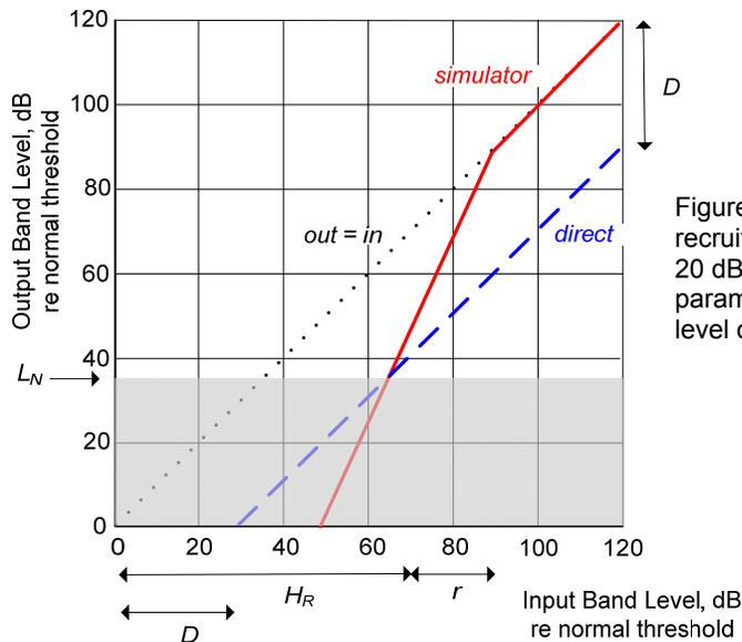
Figure 4. An example I/O plot for one simulator band with a recruiting hearing loss  $H_R = 70$  dB, recruitment range  $r = 20$  dB, and direct-path attenuation  $D = 30$  dB. These parameter values result in a direct-path-masking noise level of  $L_N = 34$  dB.
