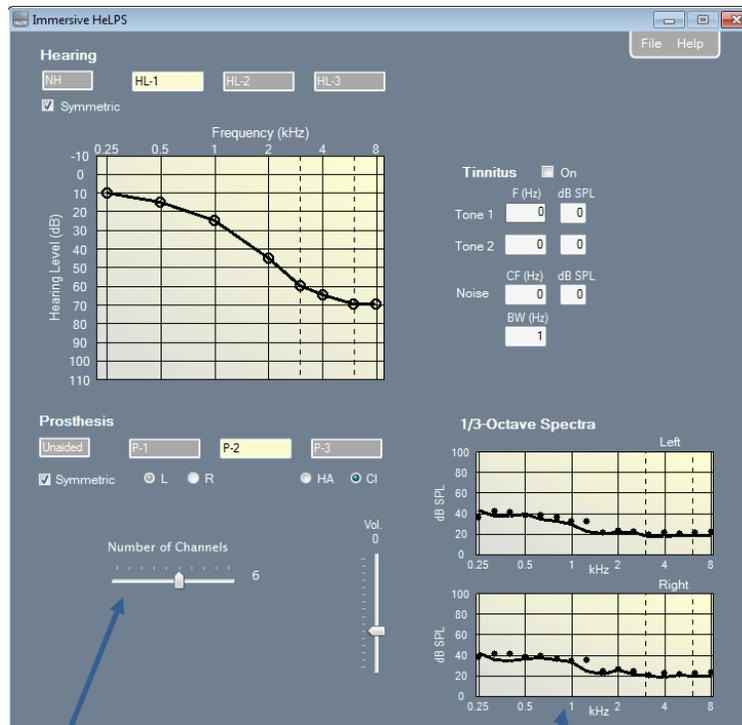
The only controls for a cochlear implant simulation are the number of channels and overall volume.
