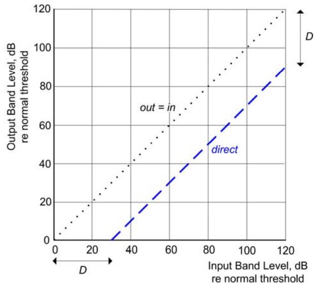
Figure 3. An example I/O plot for one simulator band showing the direct path component at  $D = 30$  dB.
