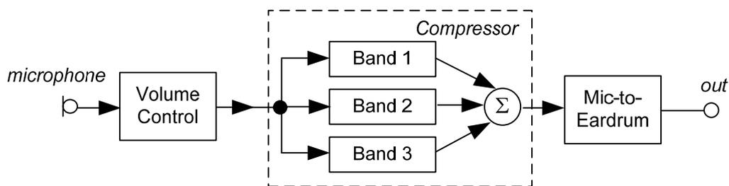
Figure 6. Block diagram of the prototype hearing aid implemented by HeLPS.
