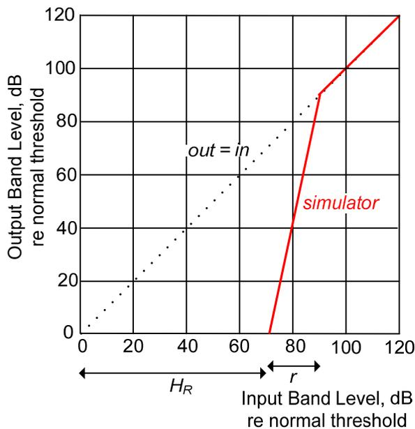
Figure 1. Example I/O plot for one simulator band showing a recruiting hearing loss  $H_R = 70$  dB with a recruitment range  $r = 20$  dB.
